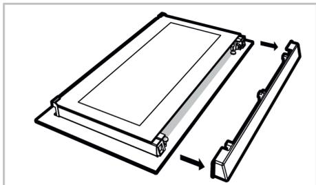
3. As shown in the figure, gently lift the innermost glass (1) towards “A” and then, remove it by pulling towards “B”.
