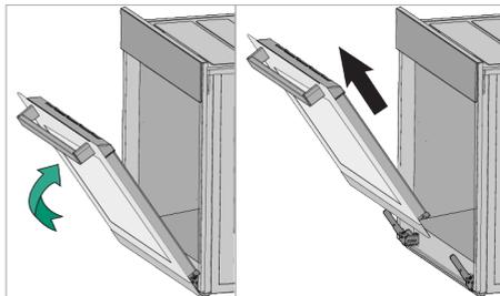
8. Pull the removed door upwards to release it from the right and left hinges and remove it.
