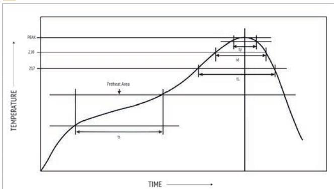
Only 1 reflow soldering cycle allowed. All temperatures are measured on the topside of the Al-can.
