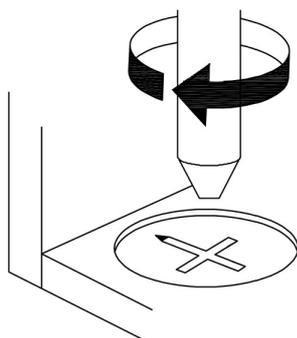
**EN\_**Turn cam lock clockwise to tighten.
