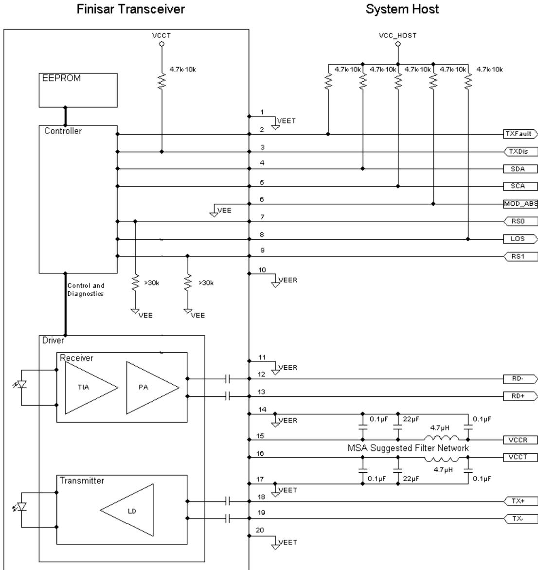
**Figure 6-Host-Module Interface**
