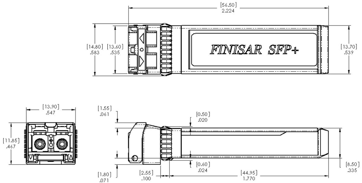
**Figure 2. FTLX1471D3BCL Mechanical Dimensions.**
