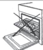
If the grease falls down into the oven burner it could inflame.
