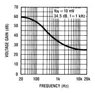
Figure 29. NAB Preamp Voltage Gain vs Frequency
