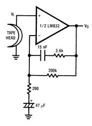
$A_V = 34.5$  F = 1 kHz  $E_n = 0.38 \text{ }\mu\text{V}$  A Weighted
