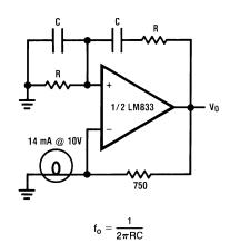
Figure 32. Sine Wave Oscillator
