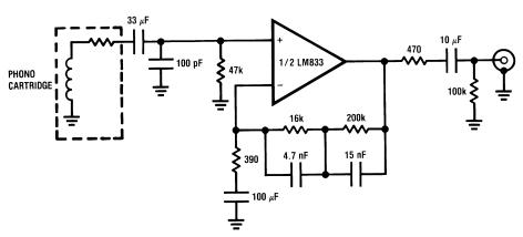
$\begin{array}{l} A_{v}=35~\text{dB}\\ E_{n}=0.33~\mu\text{V}\\ \text{S/N}=90~\text{dB}\\ f=1~\text{kHz}\\ \text{A Weighted}, \text{ V}_{\text{IN}}=10~\text{mV}\\ @f=1~\text{kHz} \end{array}$
