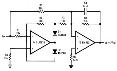
Figure 36. AC/DC Converter
