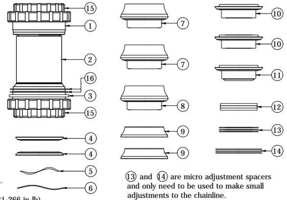
⑬ and ⑭ are micro adjustment spacers and only need to be used to make small adjustments to the chainline.
