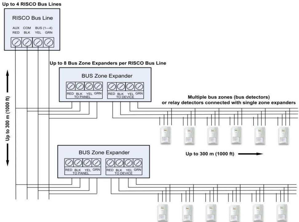
➤ **To connect multiple bus detectors to bus lines using Bus Zone Expander(s):**
