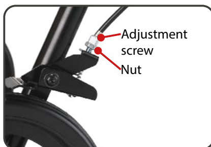
Illustration 7. Brake adjustment.
