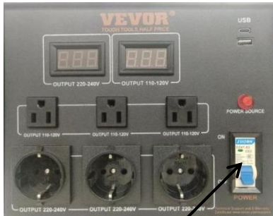
Power switch (Air switch)
