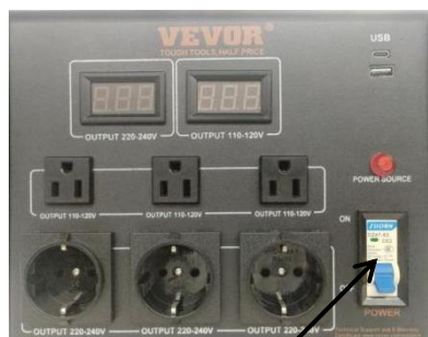
Power switch ( Air switch )
