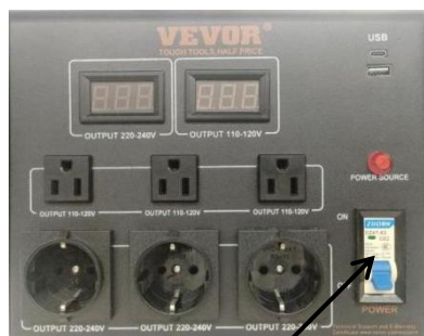
Power switch ( Air switch )
