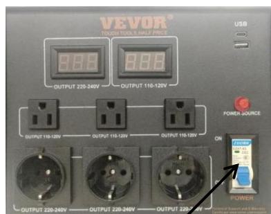
Power switch ( Air switch )
