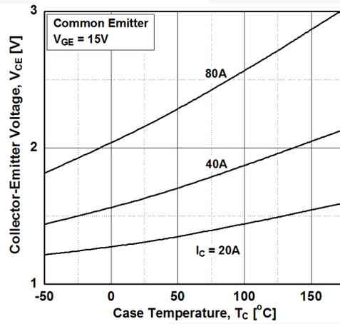
Figure 5. Saturation Voltage vs. Vge
