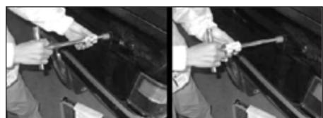
7. Remove the glue residue from the car body by spraying it with glue remover and then gently tear off by means of a scraper.
