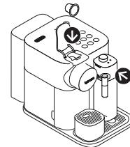
**4** Press the button relative to the desired milk-based beverage. See page 15 for further information on each milk-based beverage.
