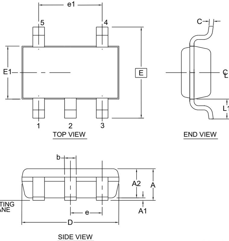
1. Dimension D does not include mold flash, protrusions or gate burrs. Mold flash, protrusions or gate burrs shall not exceed 0.15 mm per end. Dimension E1 does not include interlead flash or protrusion. Interlead flash or protrusion shall not exceed 0.15 mm per side.
