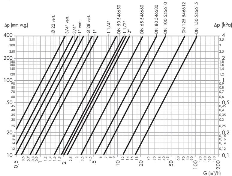
The maximum recommended speed of the medium inside the pipe is 1,2 m/s. The following table shows the maximum flow rates in order to meet this requirement.
