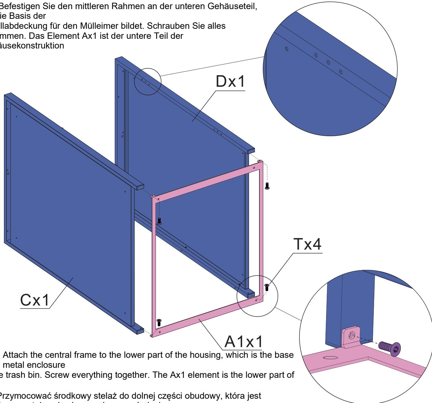
**ENG:** Attach the central frame to the lower part of the housing, which is the base of the metal enclosure for the trash bin. Screw everything together. The Ax1 element is the lower part of
