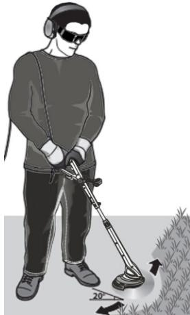
Effective mowing of the grass with the device is possible only if the grass not higher than 15 cm. Keep the grass trimmer away from hard objects. When the string or blade comes into contact with a hard object, the string or blade may break. Stones can be thrown away and hit the surrounding objects at high speed causing damage. It is prohibited to use the device without a safety cover. When using the trimmer, remember to maintain proper body posture during work.
