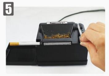
Press the lever fully down to start tube filling.
