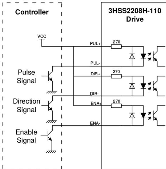
Fig. 3 Connections to common anode
