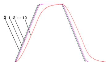
**P20 User-defined Micro Steps** User can set the micro steps according the specific situation, the actual micro steps = the set value  $\times$  50.
