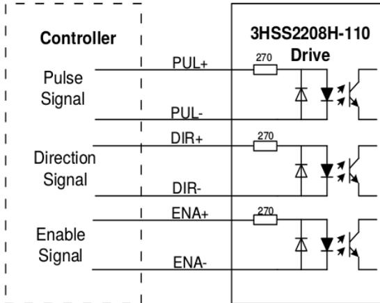
Fig. 2 Connections to differential signals
