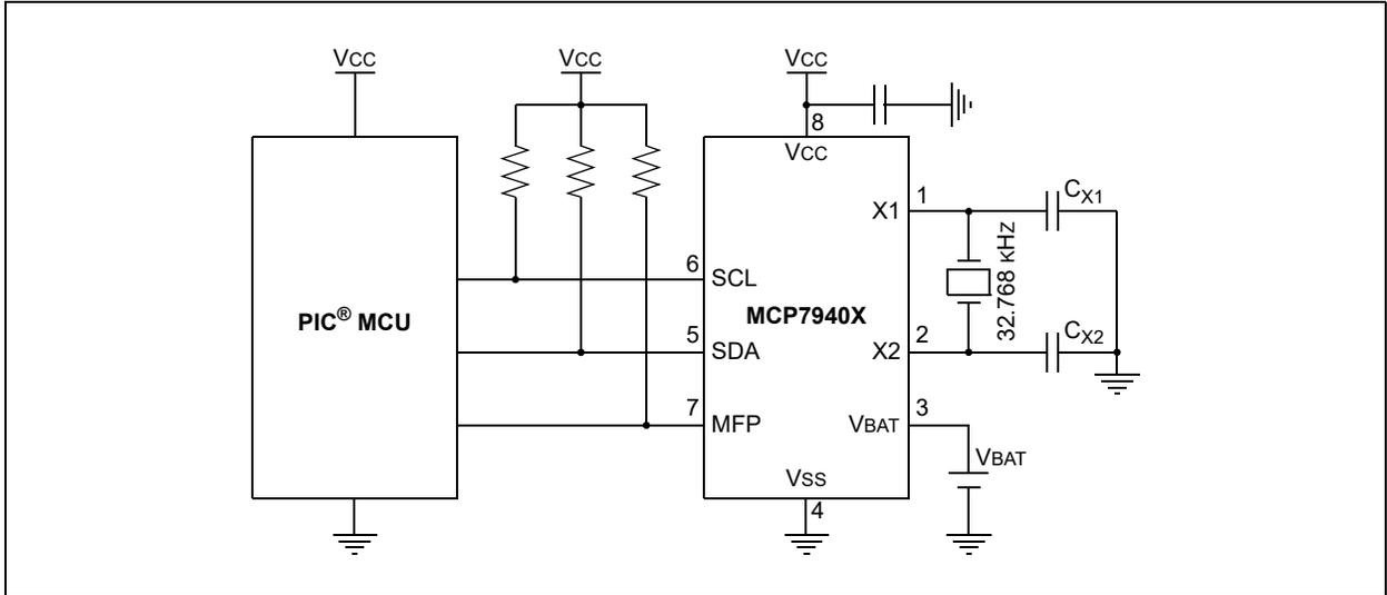
**FIGURE 1-2: BLOCK DIAGRAM**
