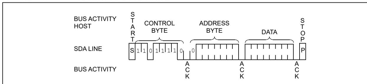
**FIGURE 6-2: SRAM/RTCC SEQUENTIAL WRITE**
