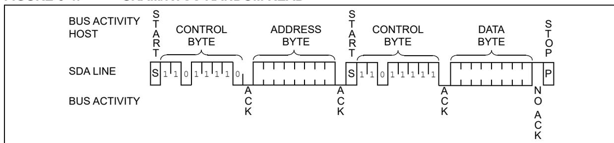
**FIGURE 6-5: SRAM/RTCC SEQUENTIAL READ**
