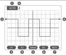
①Trigger mode indicator icon, Auto means automatic trigger, Single means single trigger, Normal means normal trigger.
