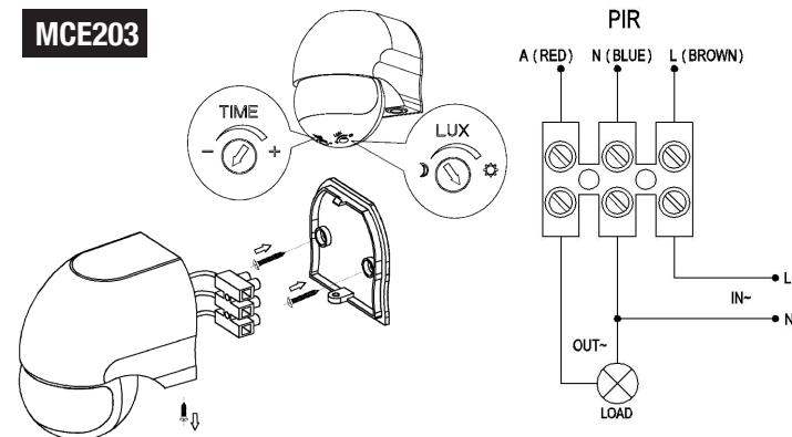
EN Infrared motion sensor
