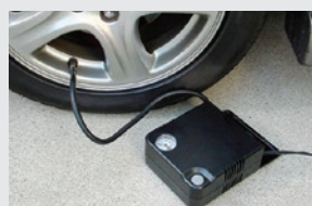
STEP2 Fill up with air by air compressor
