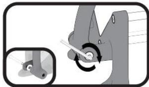
Make sure the washers have been located inside of connecting arm then insert the duel screw into holes and tight them with Allen wrench
