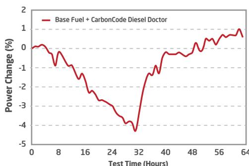
DW10 Injector "Deposit Reduction Test"
