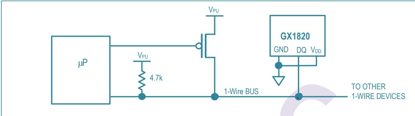
Figure 5. Powering the GX1820 with an External Supply
