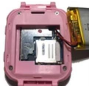
6. Slide left to lock the slot
