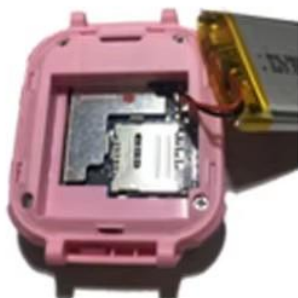
3. Slide right to open the slot
