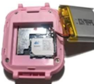
5. Insert the SIM, note the angle
