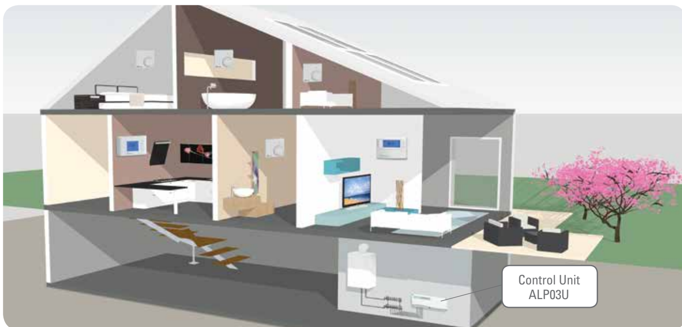
Installation example of a ALP03U with 6 room thermostats in input, 6 valves and a pump connected at the output.
