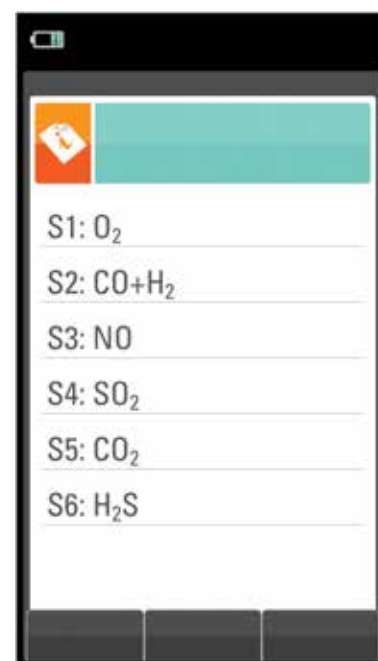
LCD screen with internal sensors arrangement
