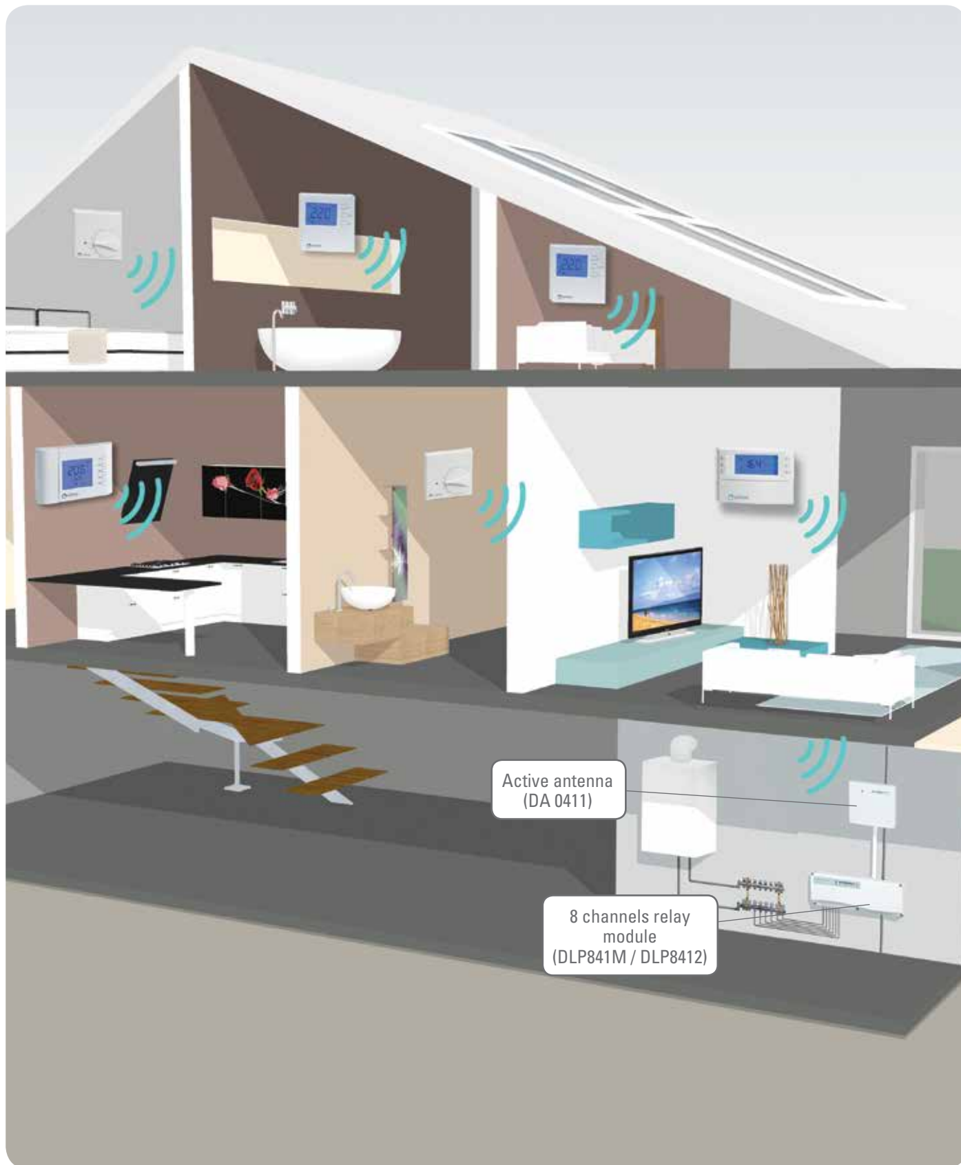
Installation example with 6 wireless thermostats, one DA 0411 active antenna and one DLP 841 2 relay module.
