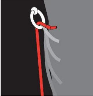
The rope which is taken in should be laid on the cliff side of the anchor point in order to avoid trapping the rope's end between the ring and the rock face.
