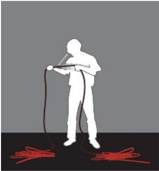
After each use, you should carefully examine your rope. To do this, run the rope through your hands meter by meter and feel for bulges, hard spots and other irregularities and look for obvious damage to the sheath. If there are significant physical irregularities, thin or open areas on the sheath, or any other signs of damage, the rope should be replaced.
