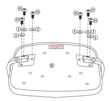
During the assembly, please first half-tighten all the screws into the holes. After all the screws are set, fully tighten them.
