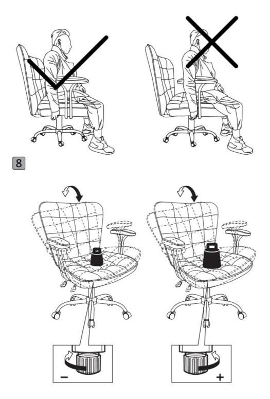
Adjust the recline angle by turning the knob located underneath the chair. Tighten the tension for heavier users by turning the knob clockwise.
