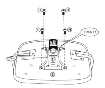
During the assembly, please first half-tighten all the screws into the holes. After all the screws are set, fully tighten them.
