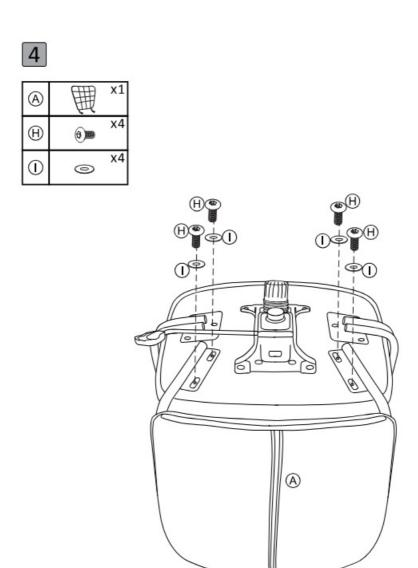
During the assembly, please first half-tighten all the screws into the holes. After all the screws are set, fully tighten them.
