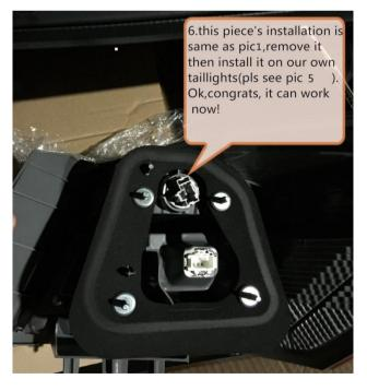
6.this piece's installation is same as step1, remove the socket then install it on our taillights' turning light wire.(see step 5)
