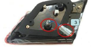
1/2/3/4.connect extension "black&blue" wire with LEFT side taillight of reversing plug.(right side taillight don't need this extension wire.)
