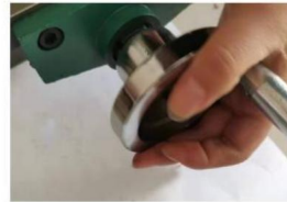
6. Align and push the handwheel in
