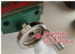
7. Push in and install the cap here
