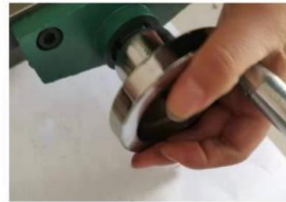
6. Align and push the handwheel in
