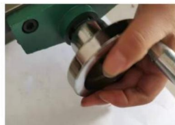
6. Align and push the handwheel in
