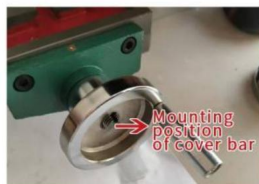
7. Push in and install the cap here
