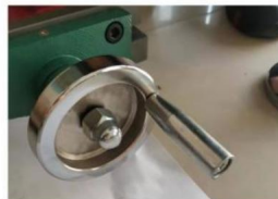
8. Cover bar is installed, handwheel is installed
