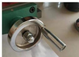
8. Cover bar is installed, handwheel is installed
