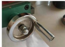
8. Cover bar is installed, handwheel is installed
