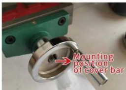
7. Push in and install the cap here
