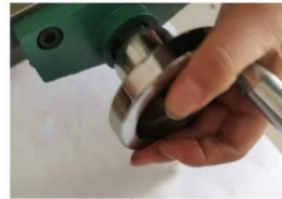
6. Align and push the handwheel in
