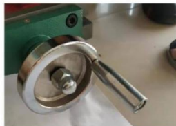
8. Cover bar is installed, handwheel is installed
