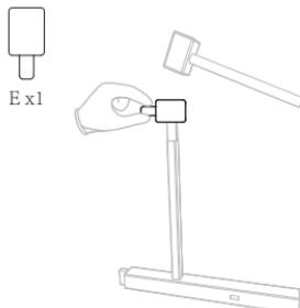
Holding the long tenon of component E, place E on top of the table component, and tap E to complete the task
