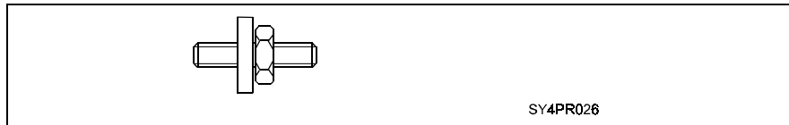
Fig. 6-7: fiber optic cable leadthroughs
