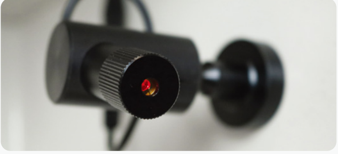
Laser Positioning Device (LD) This easy-to-install tracing tool lets you quickly determine if the design is within the hoop range.
