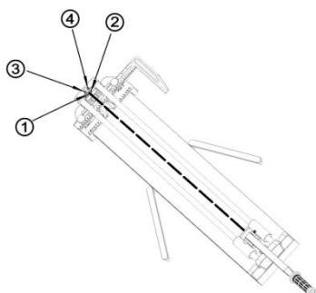
4. When the laser irradiation is too far/high, adjust the No. 3 and 4 screws clockwise.
