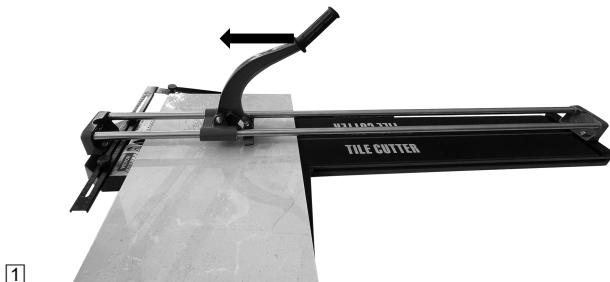
Place the cutting wheel on the rear edge of the tile.
