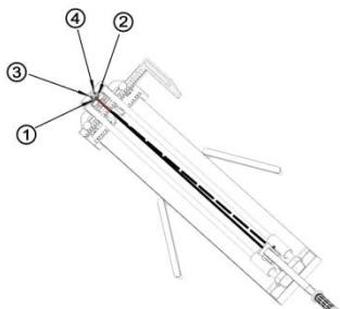
3. If the laser is biased to the right, adjust the No. 1 screw clockwise or the No. 2 screw counterclockwise.
