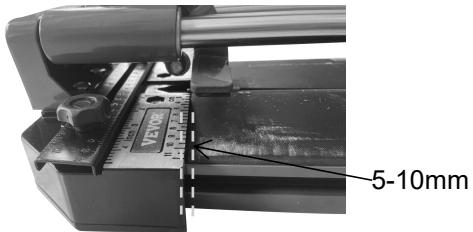
Tips: Do not put the tile too inside to make sure the scoring line is a whole line, after scoring, it is better to pull back the handle to let the breaker slightly backtrack 5-10mm,it's the best position to break the tile.
