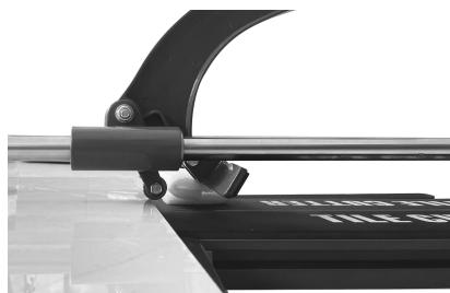
Slide the wheel forward by pushing the handle down with medium pressure.
