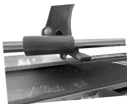
Place the cutting wheel on the rear edge of the tile.
