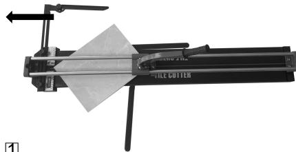
Put tile on the machine against the adjusted angle ruler.
