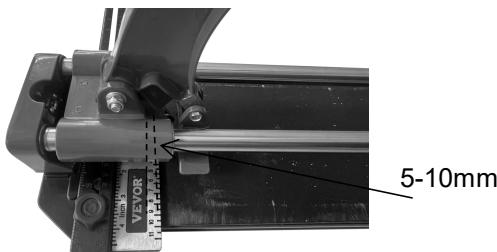
Tips: After scoring, it is better to pull back the handle to let the breaker slightly backtrack 5-10mm, which is the best position to break the tile.
