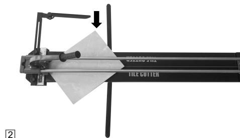
After scoring and without moving the tile position, the breaker is slightly in the front edge of the tile and front stop.
