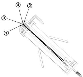
2. If the laser is biased to the left, adjust the No. 2 screw clockwise or the No. 1 screw counterclockwise.
