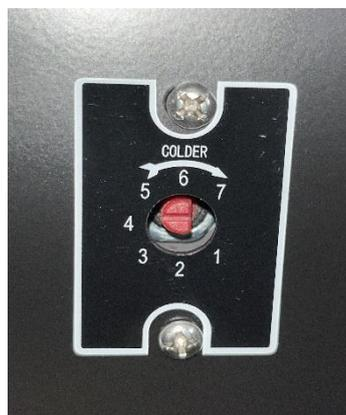
Use a flat-blade screwdriver to turn the red rotary switch to the desired level.
