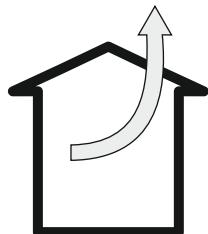
In extractor mode the air is discharged to the outside by a special conduit. Remove any charcoal filters in case if they have been installed by factory (see **Replacement of the filter**). This increases the performance of the cooker hood.
