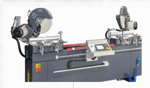
Precise and automatic positioning thanks to electronic control system and rack.
