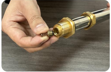
Check valve clean and check O-ring for damage.
