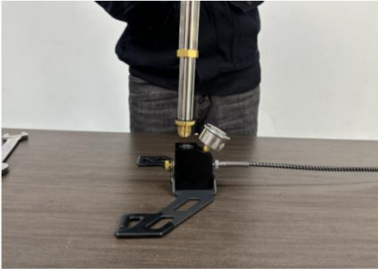
13. Screw the main body into the base to complete the installation.
