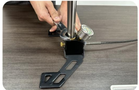
Check whether the primary piston is loose and the seal ring is damaged.
