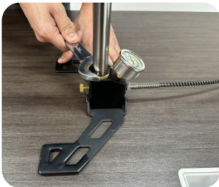
1. Release the wrench and remove the pump body.
