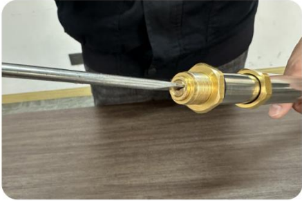
Check valve clean and check O-ring for damage.
