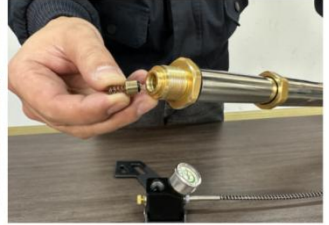
12. Install the check valve.
