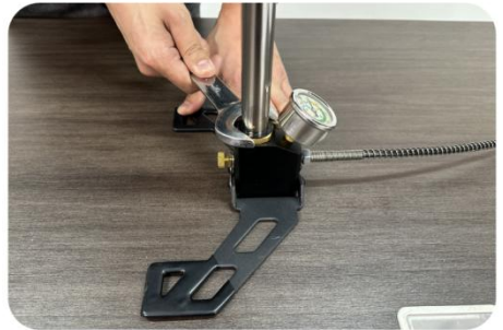
Check whether the primary piston is loose and the seal ring is damaged.
