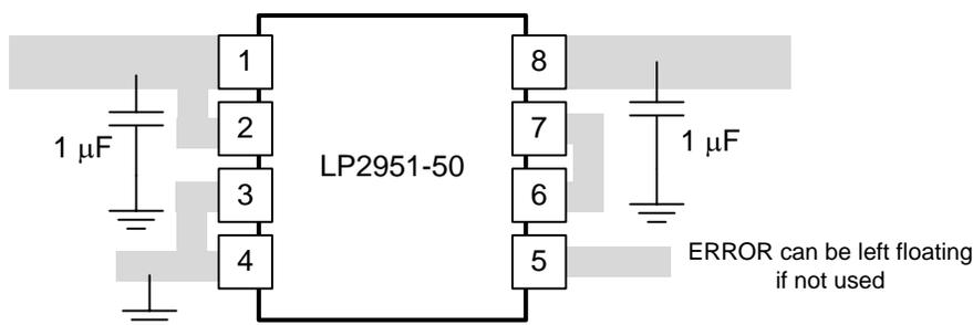
Figure 35. LP2951 Layout Example (D or P Package)
