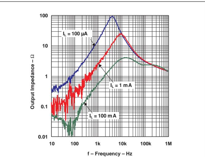
Figure 22. Output Impedance vs Frequency
