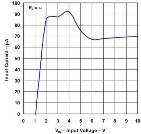
Figure 2. Input Current vs Input Voltage ( $R_L = \text{OPEN}$ )
