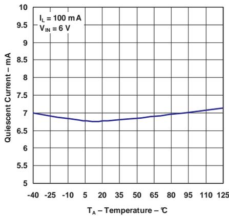
Figure 9. Quiescent Current vs Temperature ( $I_L = 100 \text{ mA}$ )
