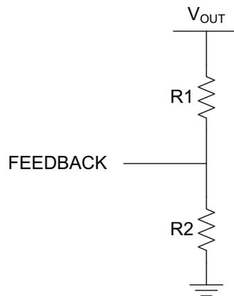
Figure 32. Adjusting the Feedback on the LP2951
