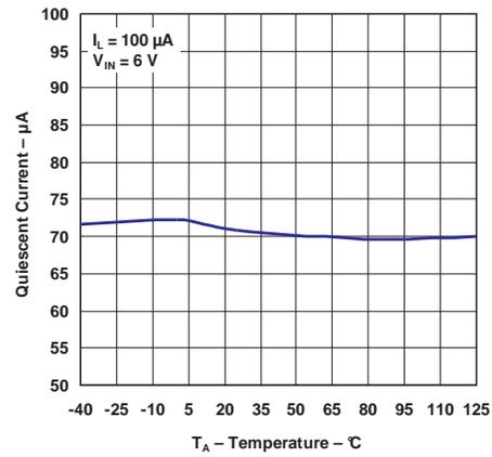
Figure 10. Quiescent Current vs Temperature ( $I_L = 100 \text{ µA}$ )
