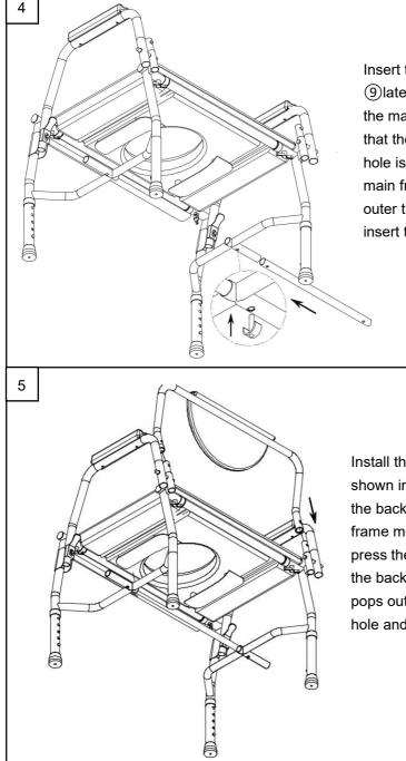
Insert the connecting tube (9) laterally on the side of the main frame mouth so that the connecting tube hole is aligned with the main frame connecting outer tube hole, and then insert the C-clip(8).
