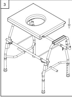
Install the seat plate, the slot on the back of the seat plate is aligned with the seat frame and then pressed down, the bottom of the seat plate buckle and the small tube of the seat frame buckle steady.
