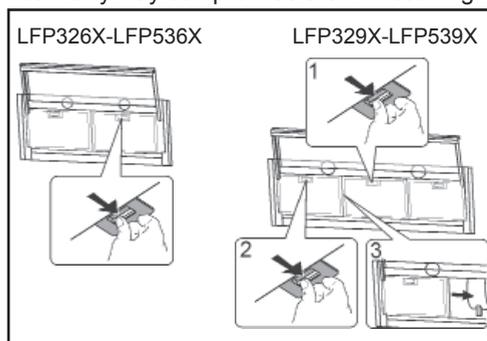
The activated charcoal filter is not washable and cannot be regenerated, and must be replaced approximately every 4 months of operation, or more frequently for particularly heavy usage.
