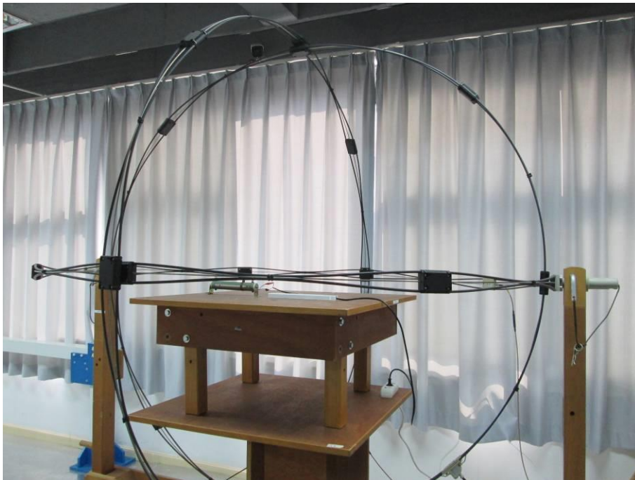
Figure B-3 Setup for Radiated Electromagnetic Disturbances
