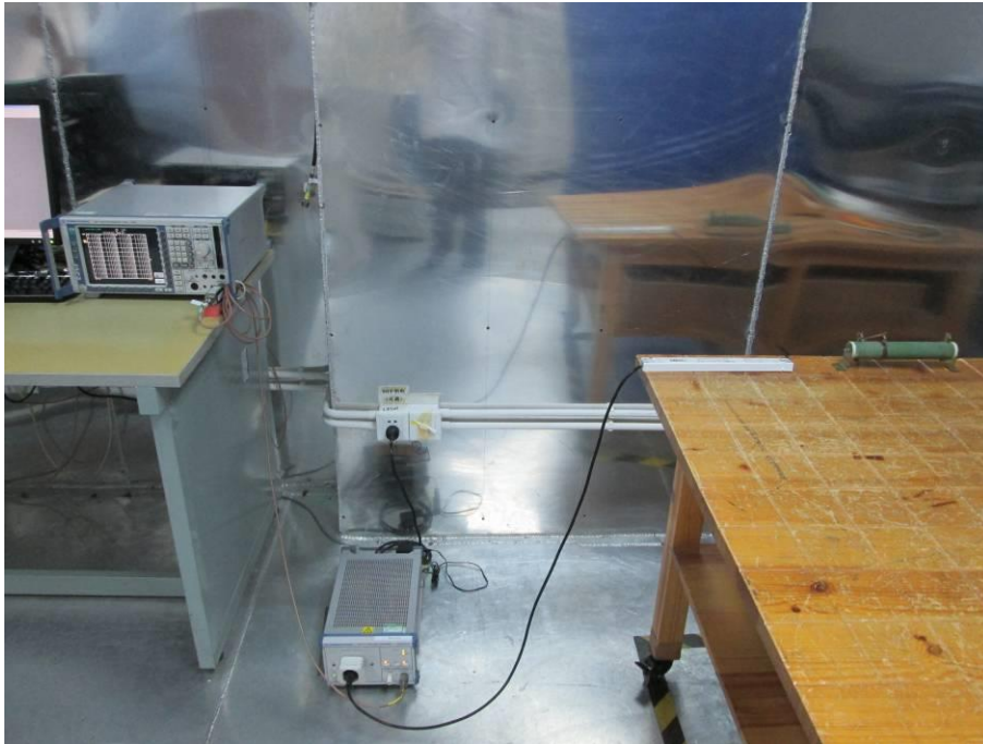
Figure B-1 Setup for Conducted Emission
