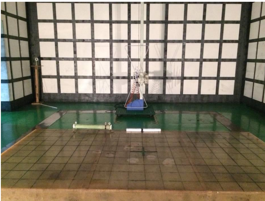
Figure B-2 Setup for Radiated Emission
