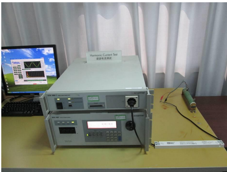
Figure B-4 Setup for Harmonic current emission & Voltage fluctuations and flicker
