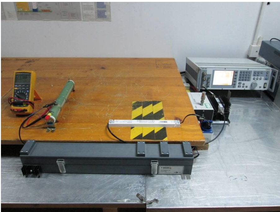
Figure B-10 Setup for Conducted immunity (DC output port)
