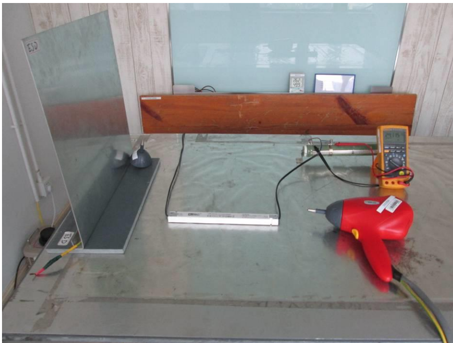
Figure B-5 Setup for Electrostatic Discharge
