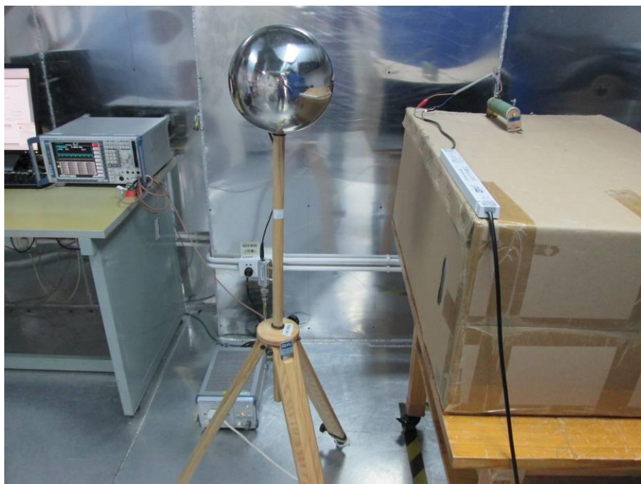
Figure B-11 Setup for Induced current density
