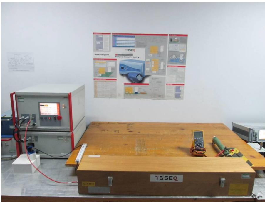
Figure B-8 Setup for Electrical Fast Transients/Bursts (DC output port)
