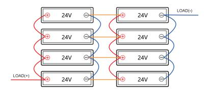
Taking a 24V100Ah battery as an example, first, four 24V100Ah batteries are connected in parallel, and then two 24V 400Ah batteries are connected in series, resulting in a battery pack with a total of 48V and 400Ah.
