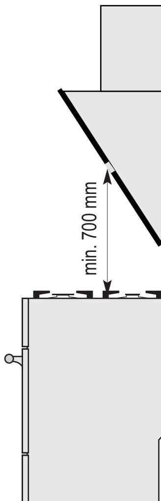
The device shall be installed at the distance of at least 650 mm above the working top of an electro and 700 mm above a gas cooker.
