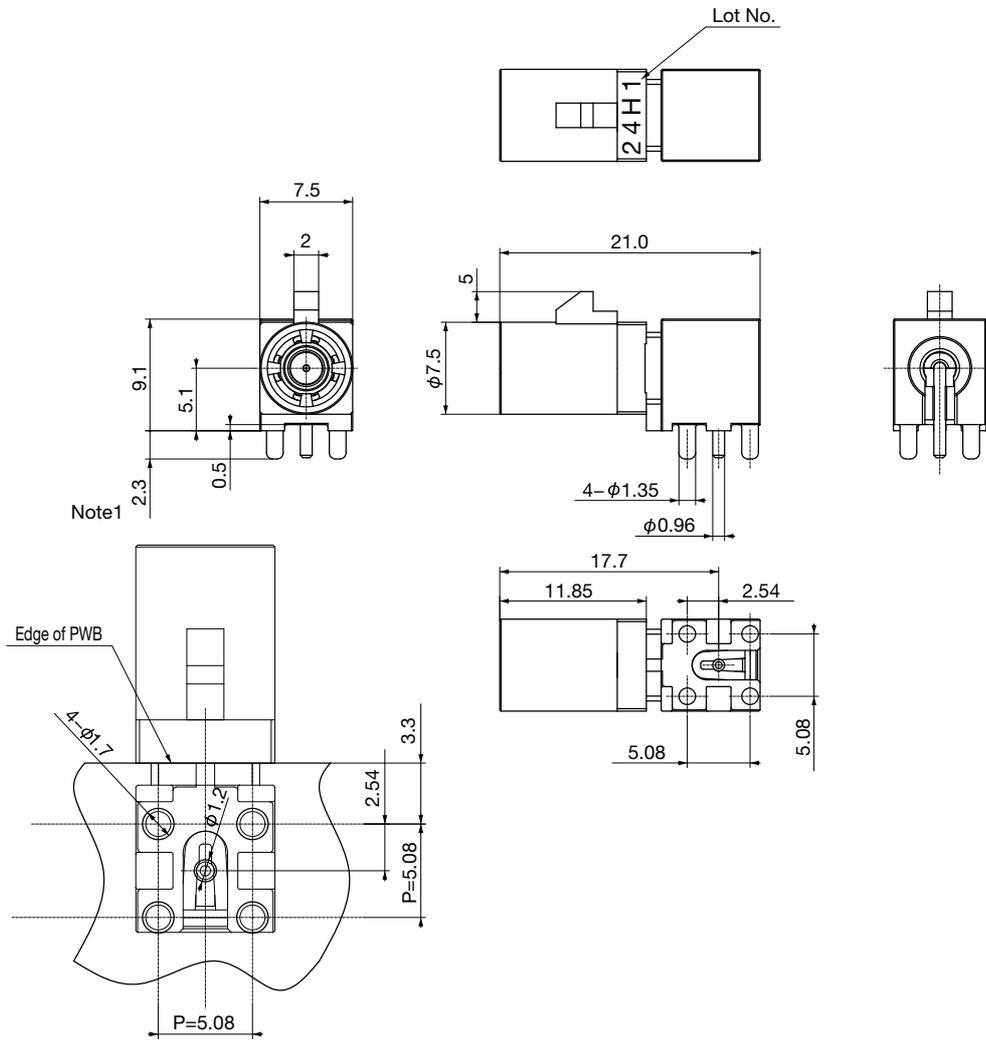
The reference PWB size. (TOLERANCE:±0.05)
