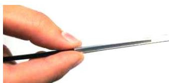
Put the fiber through the splicing tube so to protect fusion point after splicing. Make sure there is no impurity inside <sup>20</sup> the tube and keep the tube parallel with the fiber.
