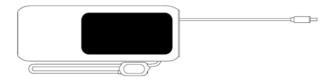
To adjust the cable, pull again, adjust to the desired length, then pull slightly (about 0.4" / 1 cm) and stop to set it in place.
