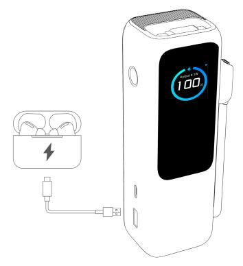
Press the power button twice to exit trickle charging mode.
