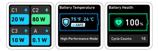
Active Cooling Mode: Displayed when the battery temperature is slightly high, reducing the power of charging or recharging to cool the power bank.
