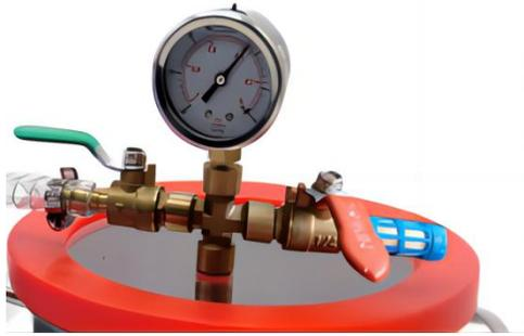
5. After the connection, start the power normally, and you can see that the pointer pressure of the vacuum gauge will rotate.
